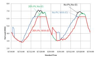
Figure 7 – Substation Load (black) with PV and Energy Storage (red), with PV (green), and Energy Storage (blue)
