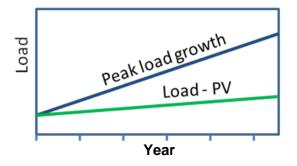
Figure 6 - Effect of PV deployment on load growth
