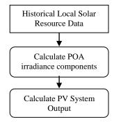
Figure 2 - Estimation of PV array Output
