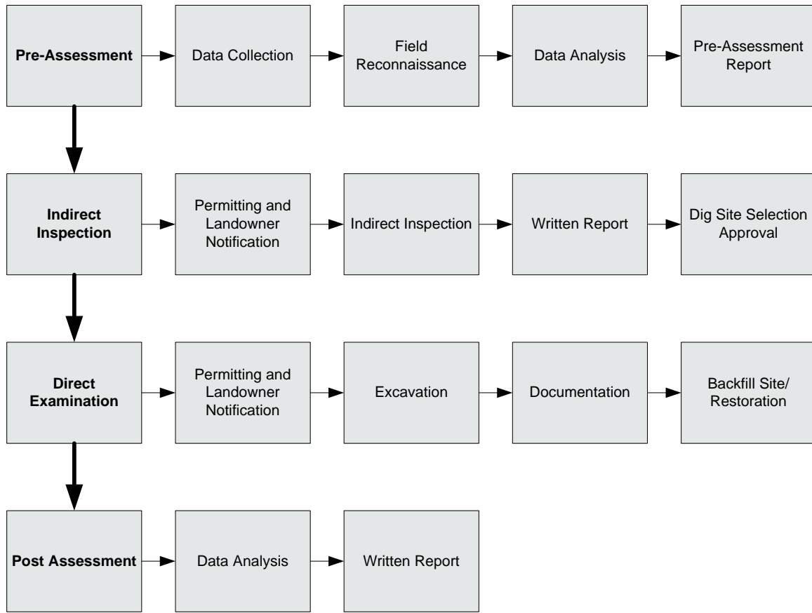
Figure 1 – ECDA Process Overview
