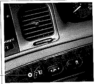
Fuel gauge and selector switch mounts flush inside every vehicle
