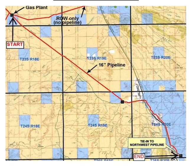
START AT GAS PLANT END AT TIE-IN TO NORTHWEST PIPELINE STEEL WITH 16 INCH DIAMETER GRAND COUNTY, UT
