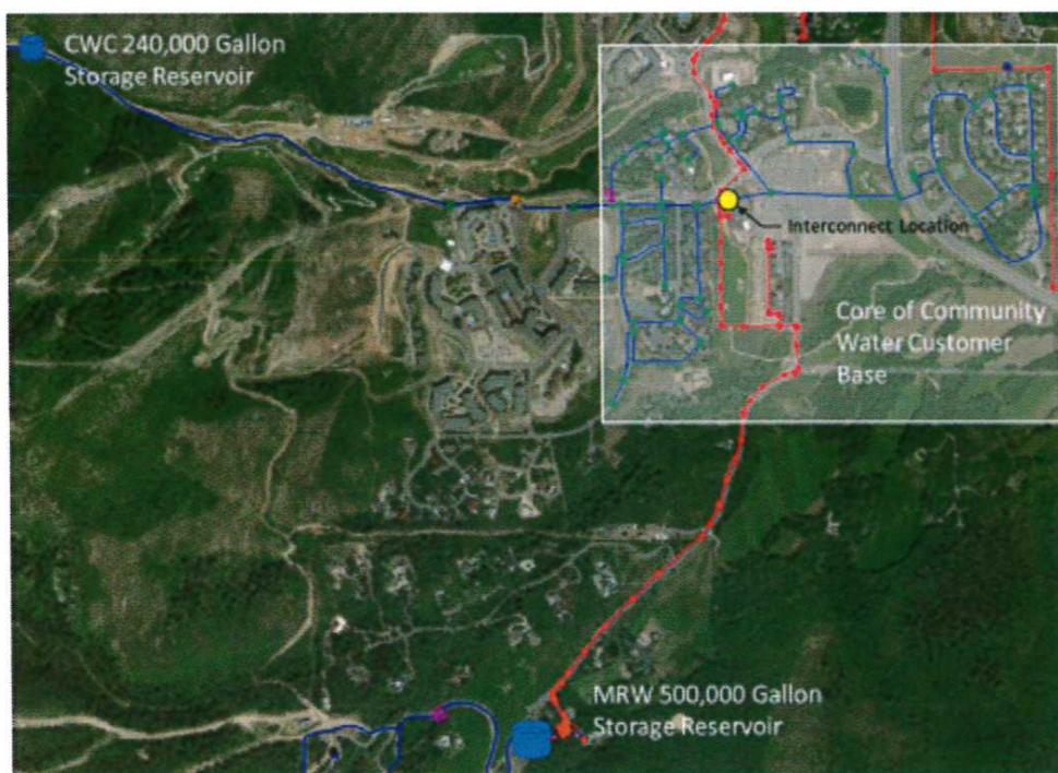
Figure 2: Overview of the layout of the MRW and CWC systems and location of the interconnect facility
