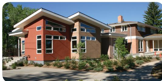
**University of Wyoming – Bim Kendall House** – The 6-kilowatt solar system will offset 30 percent of the building's electricity use. The renovated 1950s building is used by students, faculty and staff of the Environment and Natural Resources program.
