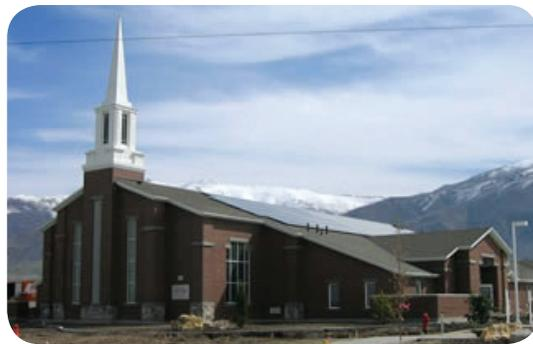
**LDS Church meetinghouse** – This 35-kilowatt solar project located in Farmington, Utah features 156 rooftop solar panels and a performance monitor display in the building library to show members the generated energy levels, power usage and power savings. This is the first solar-powered LDS meetinghouse in North America. Estimates suggest the solar panel system will generate enough electricity to meet the meetinghouse's needs.
