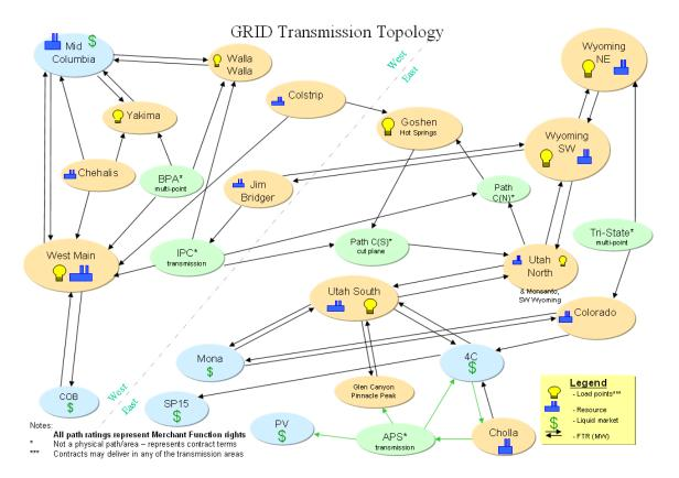
Based on the transmission rights for the Company's share of the Colstrip and Jim Bridger plants, below are the transmission topologies for the East and West.
