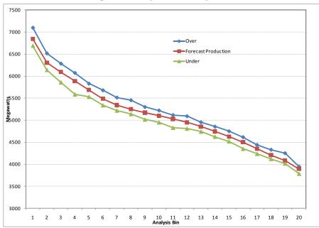
Figure 11. Example of bin analysis for load following reserve service from wind variability at the 1,372 MW penetration level for the West Balancing Authority Area (May 2007-2009).
