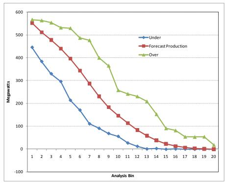
Figure 12. Example of bin analysis for load following reserve service from wind variability at the 1,372 MW penetration level for the East Balancing Authority Area (May 2007-2009).
