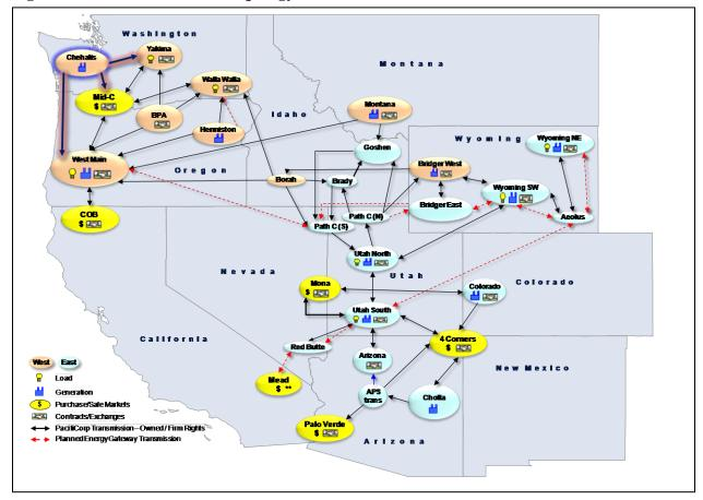
Figure 13. PaR transmission topology.
