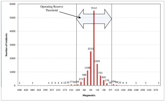
Figure 8. Load Regulation errors plotted for the Mays of the Initial Term.
