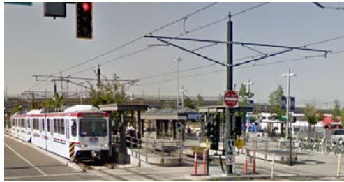
TRAX line, predictable MW-level pulsed load
