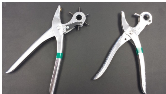
Figure 13—Two Styles of Leather-Punch Tools for Creating Additional Holes for Pinning
