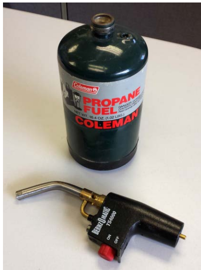
Figure 5—Propane Torch for the Installation of Heat-Shrink Tape
