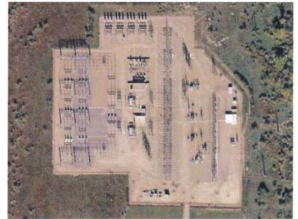
Above: Camp Williams Substation. 345 kV to 138 kV, 138 kV to 12.5 kV. Below: 90th South Substation 345 kV to 138 kV, 138 kV to 46 kV, 138 kV to 12.5 kV.
