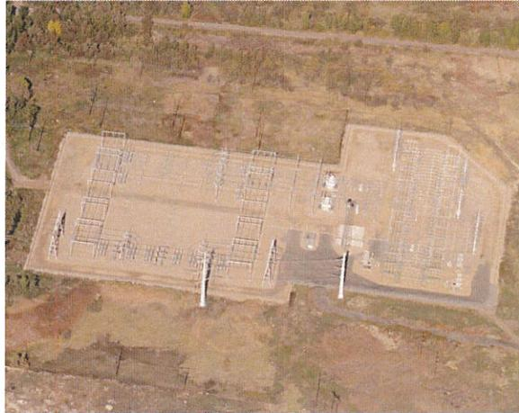
Midvalley Substation. 345 kV to 138 kV
