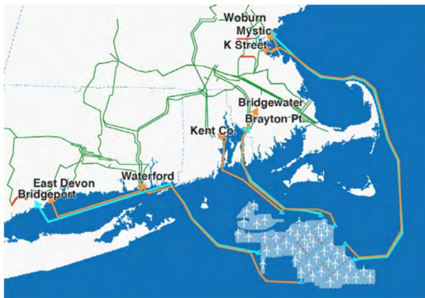
Figure B-1. Anbaric/Brattle study showing offshore HVDC grid design to enable 8.6 GW of wind without requiring major onshore grid updates.
