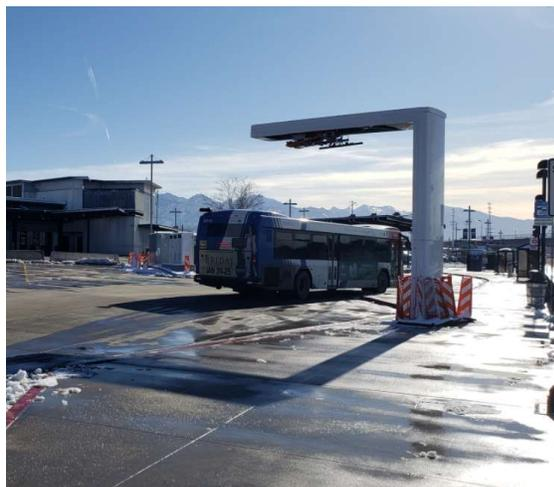
**Figure 37 - UTA electric bus at overhead charge station**
