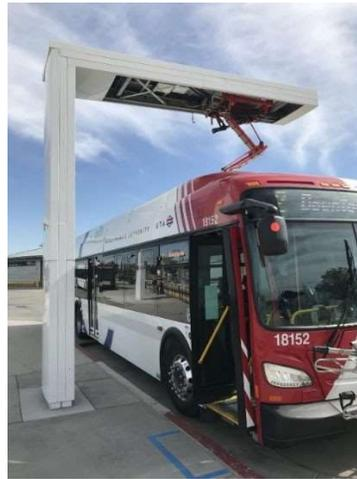
**Figure 1 - Pantograph
