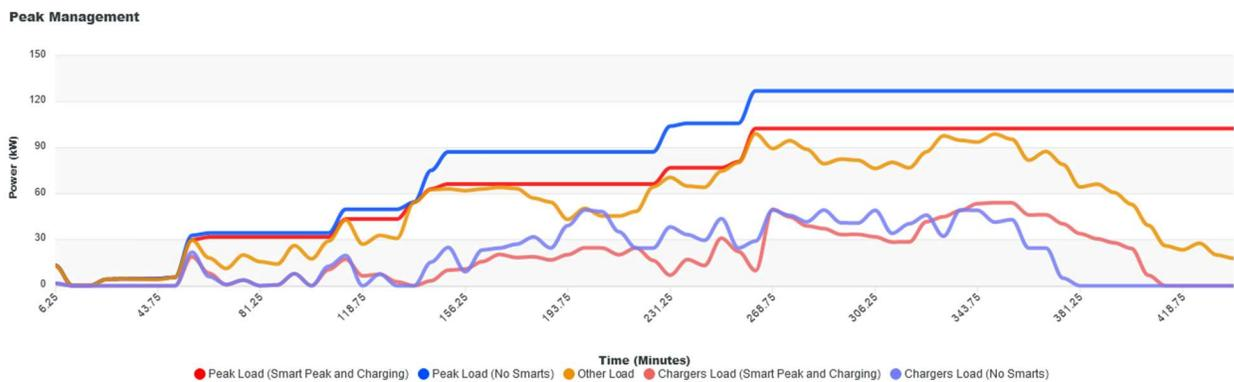
**Figure 16 - Illustrates Smart Peak Management Combined with Smart Charging**
