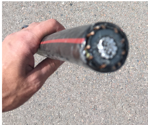
High voltage cable not encased in conduit - like the one used in the Rose canyon line extension - the same cable pictured in the original complaint.
