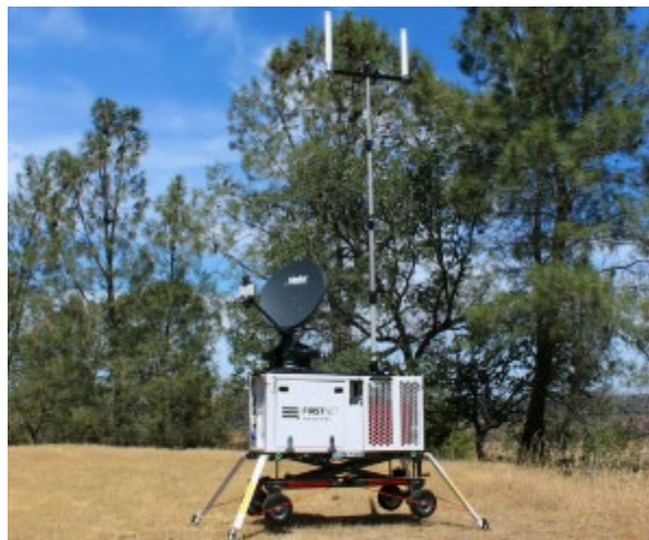
Figure 37: Rapidly Deployable Cell on Wheels
