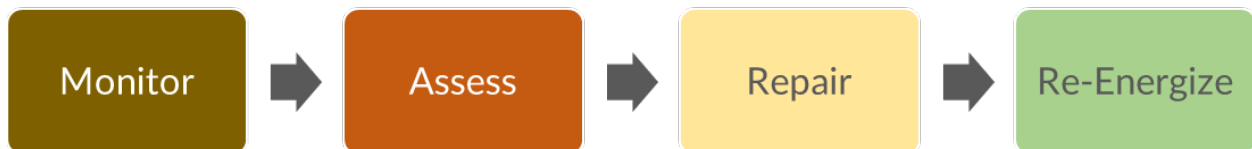
Figure 41: General Re-Energization Process
