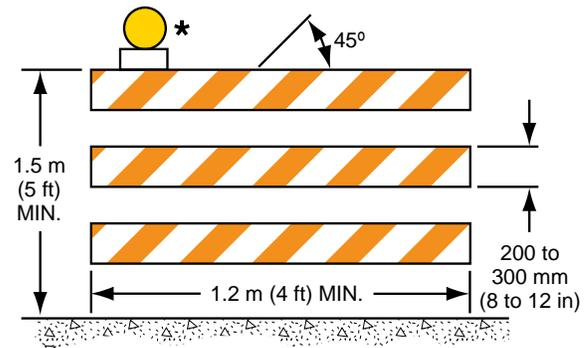
\* Rail stripe widths shall be 150 millimeters (mm) (6 inches (in.)), except that 100-mm (4-in.) wide stripes may be used if rail lengths are less than 900 mm (36 in.). The sides of barricades facing traffic shall have retroreflective rail faces.
