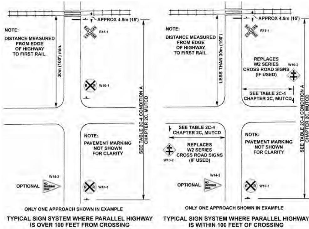
Figure 14. Substandard Clear Storage Distance
