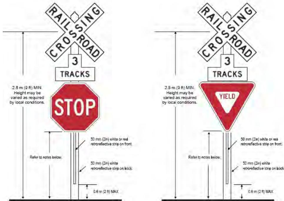
\* Note: 1.2-meter (4-foot) minimum for installations of STOP or YIELD sign on existing crossbuck sign support; 2.1-meter (7-foot) minimum in areas with pedestrian movements or parking.
