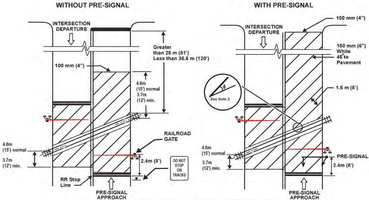
Note: 1. Pavement markings to be installed only on approaches to intersections controlled by traffic signals which are interconnected with the railroad warning signals.
