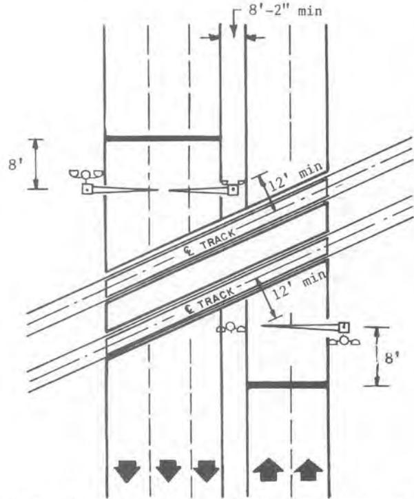
Note: The median width of 8'2" is an operational requirement and is not an AASHTO recommendation for median width.
