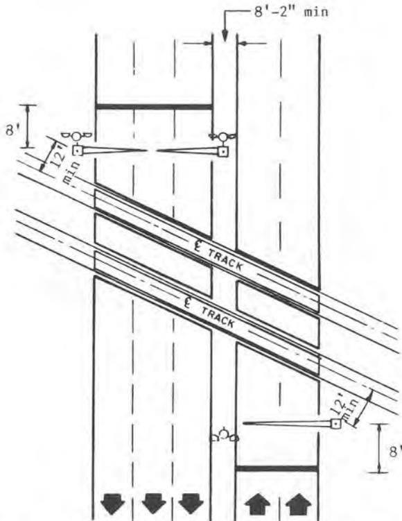
Note: The median width of 8'2" is an operational requirement and is not an AASHTO recommendation for median width.
