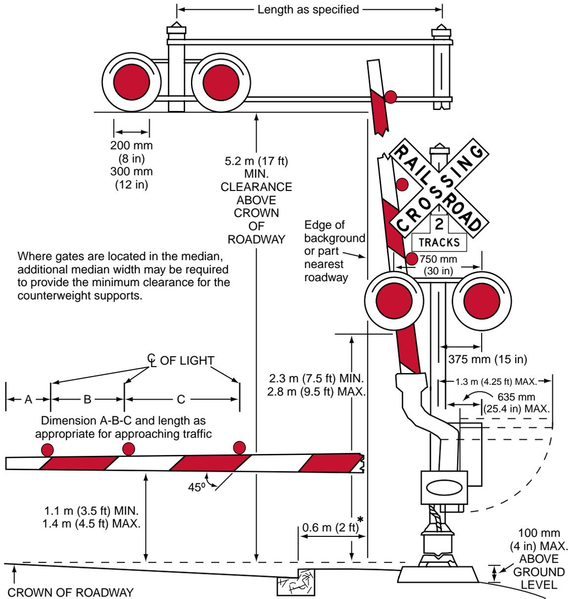
\* For locating this reference line at other than curb section installation, see Section 8D.01.
