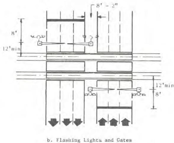
Note: The median width of 8'2" is an operation requirement and is not an AASHTO recommendation for median width.
