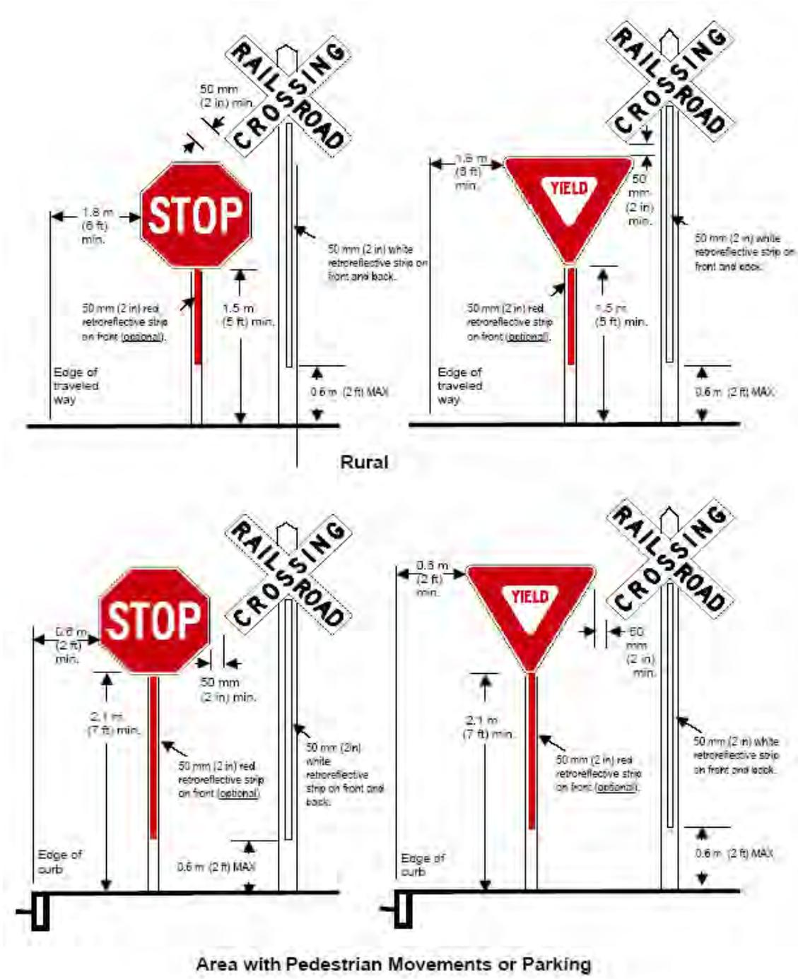
\* Note: Place face of signs in the same plane and the YIELD or STOP sign closest to the traveled way; 50-millimeter (2-inch) minimum separation between the edge of the crossbuck sign and the edge of YIELD or STOP sign.
