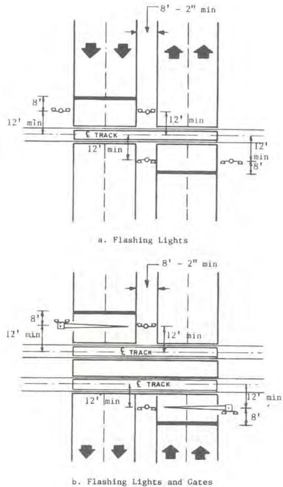
Note: The median width of 8'2" is an operation requirement and is not an AASHTO recommendation for median width.
