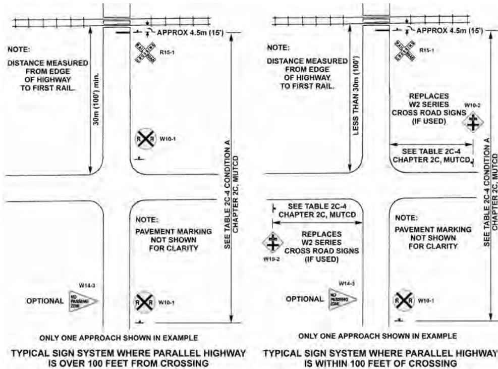
Figure 14. Substandard Clear Storage Distance
