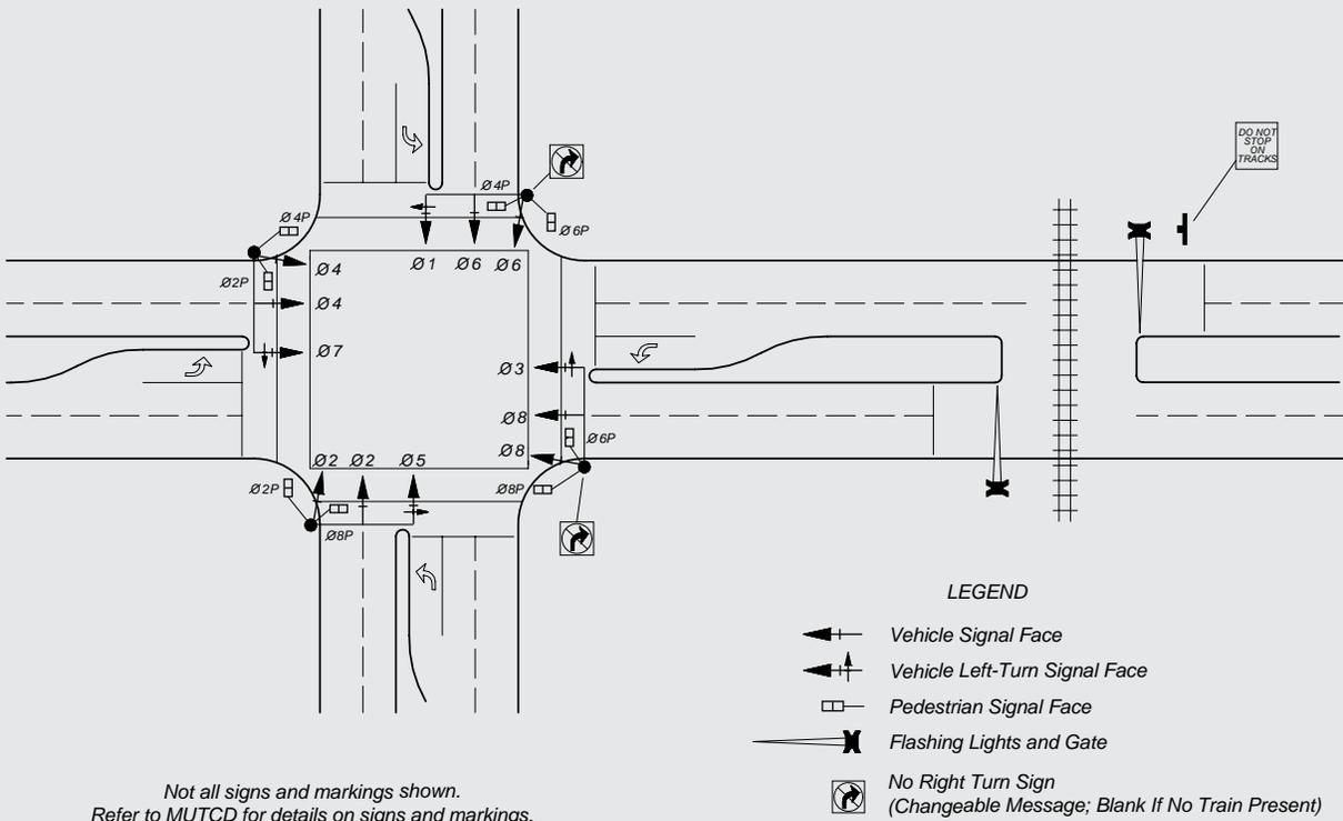
**Traffic approaching the tracks from the signalized intersection.** The placement of train detection equipment should be governed by the preemption time required to clear the queues. This time should take into account the critical or design vehicle and should be sufficient for this vehicle to clear the intersection safely before the arrival of the train.
