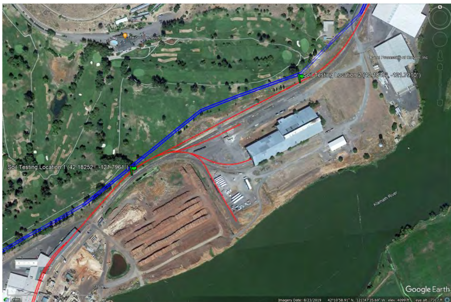
Figure 18: Soil Resistivity Measurement Locations Along Shared Corridor
