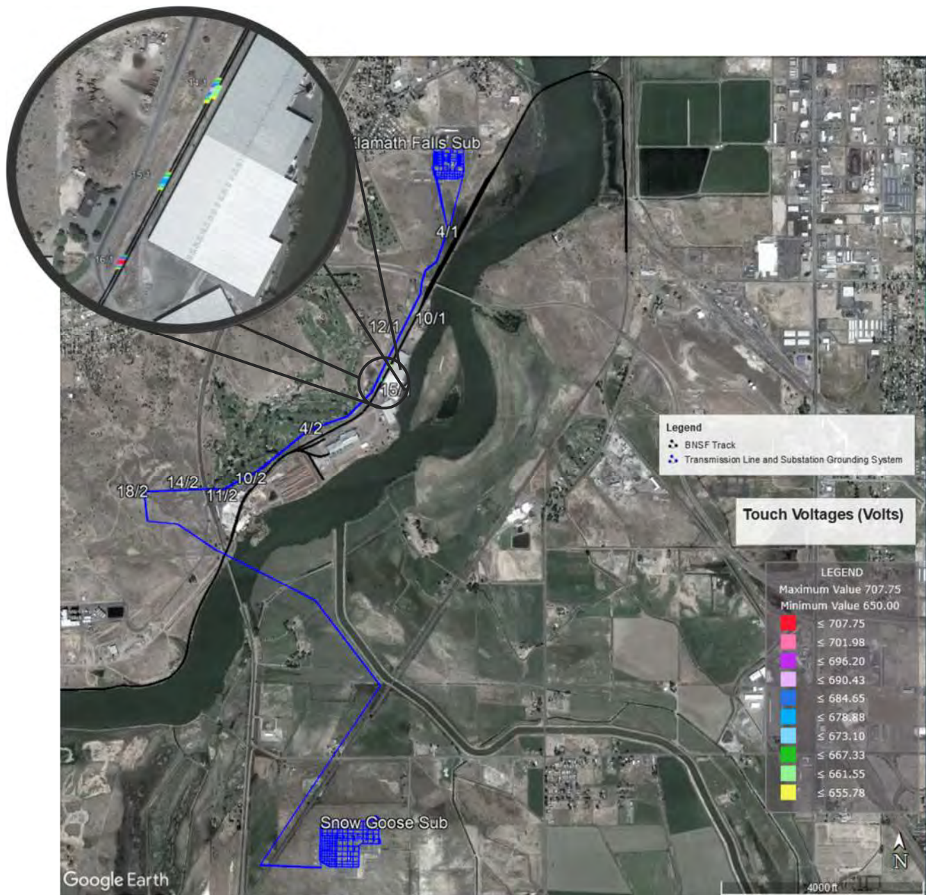
Figure 31: Rail Touch Voltages - Faulted 230 kV Structure 14/1 - Future with 230 kV Condition
