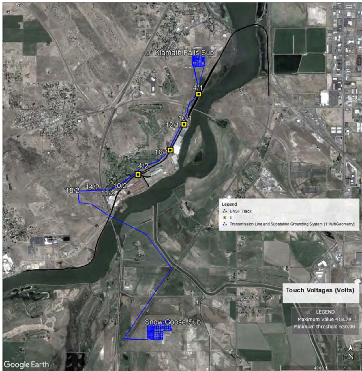
Figure 37: Mitigated Rail Touch Voltages - Faulted 69 kV Structure 9/1 - Future with 230 kV Configuration
