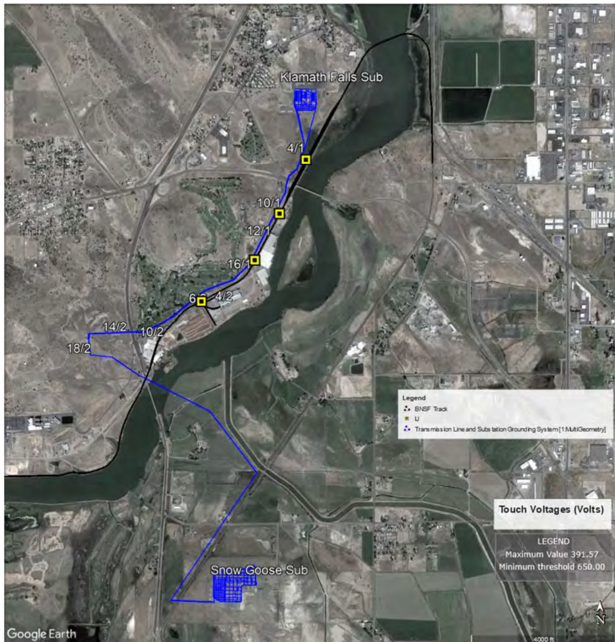
Figure 40: Mitigated Rail Touch Voltages - Faulted 230 kV Structure 9/1 - Future with 230 kV Configuration
