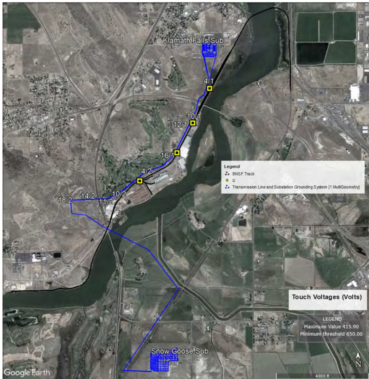
Figure 35: Mitigated Rail Touch Voltages - Faulted 69 kV Structure 4/1 - Future with 230 kV Configuration
