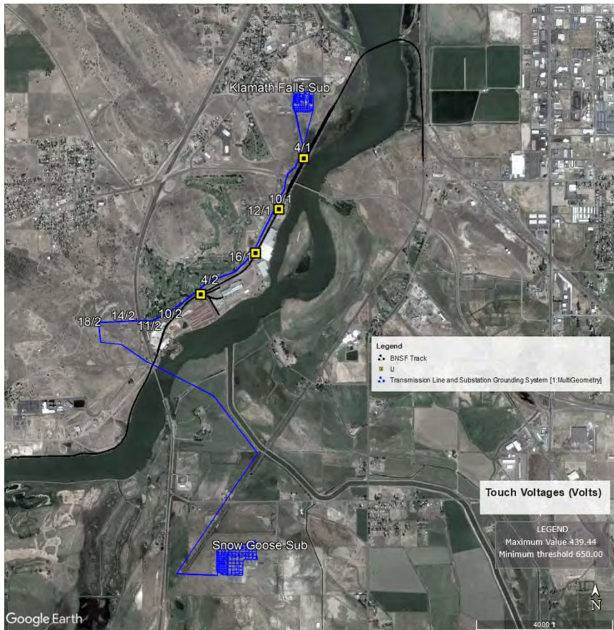
Figure 36: Mitigated Rail Touch Voltages - Faulted 69 kV Structure 6/1 - Future with 230 kV Configuration
