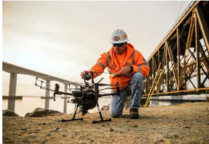
Photo credit: UP website – UP Inspector preparing UAS for flight to inspect bridge.
