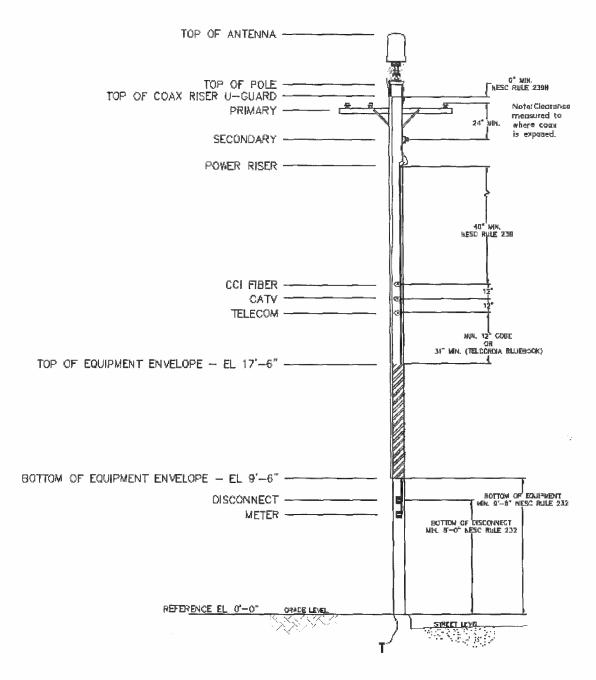
IF NO ELECTRIC UTILITY IS ATTACHED TO THE POLE (OR HAS AN APPROVED APPLICATION TO ATTACH) THE ATTACHMENT MAY ALTERNATIVELY BE LOCATED ON THE POLE TOP WITH NO BOLTS OR SCREWS IN THE TOP 12 INCHES OF THE POLE. ALL ATTACHMENTS MUST MEET NESC, FCC, STATE AND LOCAL REQUIREMENTS.
