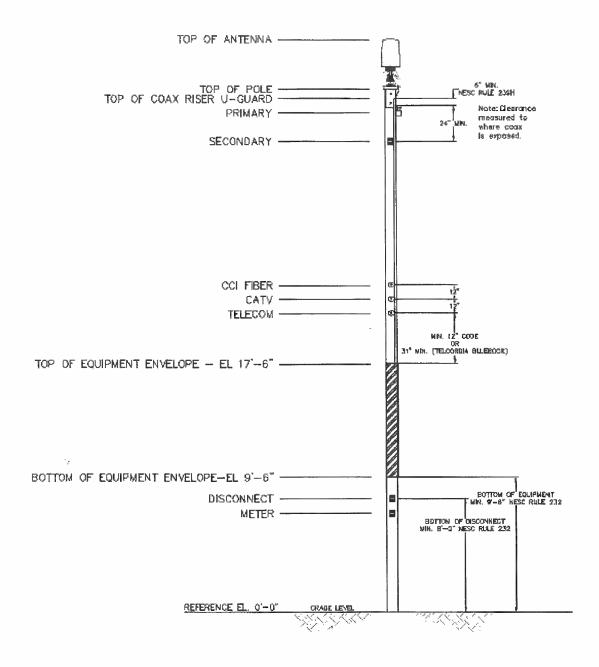
IF NO ELECTRIC UTILITY IS ATTACHED TO THE POLE (OR HAS AN APPROVED APPLICATION TO ATTACH) THE ATTACHMENT MAY ALTERNATIVELY BE LOCATED ON THE POLE TOP WITH NO BOLTS OR SCREWS IN THE TOP 12 INCHES OF THE POLE. ALL ATTACHMENTS MUST MEET NESC, FCC, STATE AND LOCAL REQUIREMENTS.
