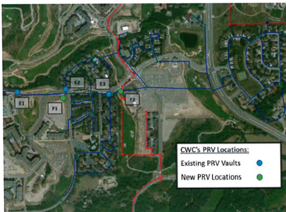
Figure 6: Overview of the CWC PRV locations both current and future
